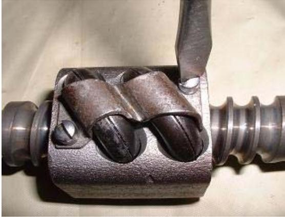
23. Install and secure ball guide clamp. Lubricate well with a good gearbox lube. Make sure you get it in the threads and work it into the nut assembly.
