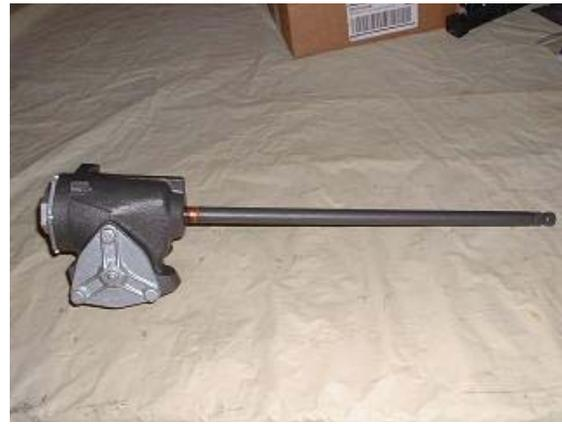
32. Now all that's left is to install the box. Be sure the box is centered (remember counting the turns?), the wheels are straight ahead and the steering wheel is centered before installing the pitman arm.
