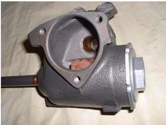
27. Install other bearing and screw cap on. In the following steps you will need to turn the shaft with a torque wrench. Gently push a socket onto the splines to torque the shaft.
