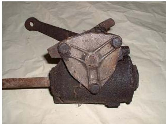
2. The adjusting screw is turned all the way in. That's not a good sign. Someone likely tried to mask worn steering components by adjusting here.
