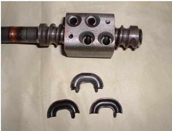
19. Notice the tabs on the end of the ball guides. If the worm nut is allowed to run all the way to the end (when assembled) it could bend these tabs.
