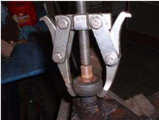
3. Use a puller and remove the pitman arm. I almost always have to apply some heat from a small propane torch to get them off.
