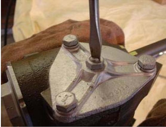
29. Center worm shaft by counting turns from end to end then turn back exactly half that number. Turn lash adjusting screw in until it just gets snug, then back off 2 or 3 turns for now.
