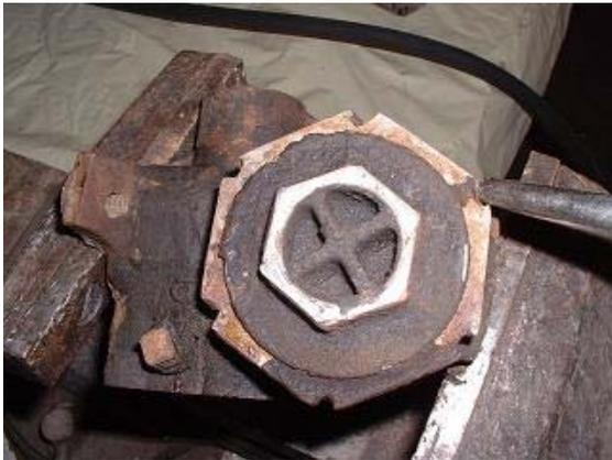
7. Next we will have to break loose the spanner nut. I don't have a tool for this so I'll just use a large punch.
