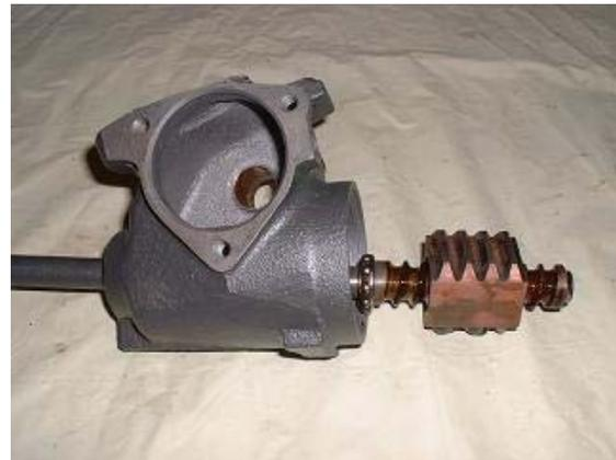
26. Pack everything with lube (not shown here for clarity), you can't get too much. Then slide bearing on shaft and insert it all into the housing.
