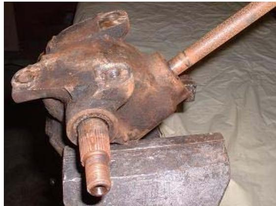
4. Scrape off the excess grease then use sand paper or emery paper to clean the shafts. This will aid in disassembly.
