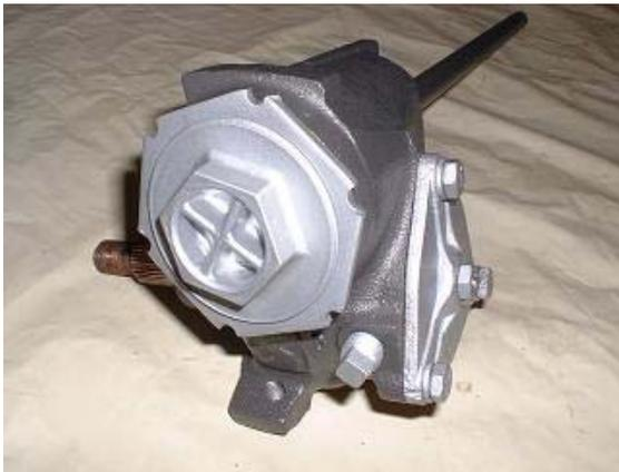
31. Now tighten pitman adjusting screw while torquing thru center for an additional 8-10 in. lbs. For example if you had 4 in. lbs. in step 30 you would need to adjust the screw until you have  $8 + 4 = 12$  min. or  $10 + 4 = 14$  max. Always make final adjustment in the clockwise direction. Tighten the small jam nut.
