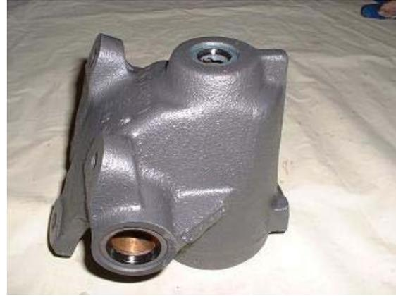
24. Drive in the new bushings and seals using the sockets you drove them out with. Lubricate the bushings and seals with gearbox lube.
