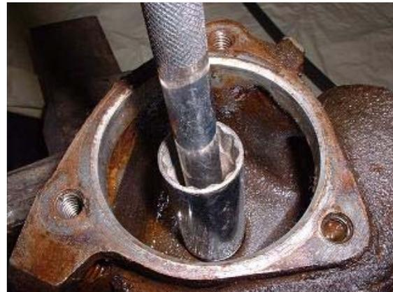
10. Use a socket to drive out the bushing and seal. Note the socket is turned around backwards. This keeps the socket from being damaged.
