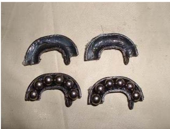
21. Smear some grease in all 4 of the guides then place 6 balls in each of 2 of the guides. Now place the guide halves together.
