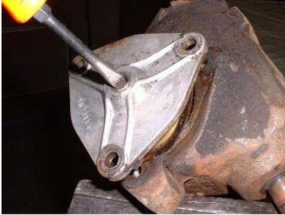
5. Remove the jam nut and the 3 screws that hold the cover. Now turn the adjusting screw all the way in and it will push the cover right off.
