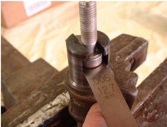
25. The manual says adjusting screw clearance should be no more than .002. This one will have to use a thicker shim (corvair.com part #CX3810).
