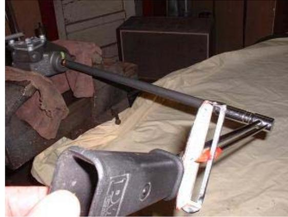
30. While turning worm shaft with a slow steady pressure slowly tighten the large worm bearing adjusting nut until you get 3 1/2 to 4 1/4 inch pounds torque. Now lock down the large jam nut.
