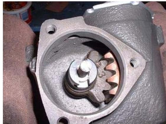
28. Install pitman shaft being careful to center gears. Install adjusting nut and shim then install bearing cap by turning screw counter clockwise and backing it into the cap just as it was removed.
