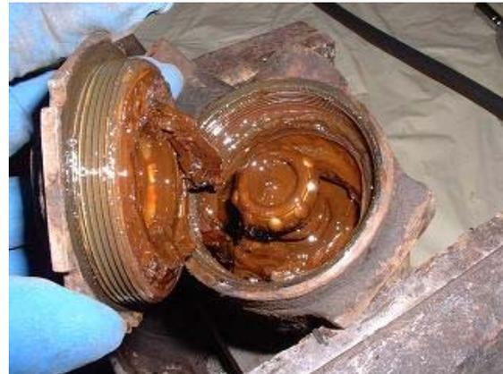
8. Remove the nut which will expose the worm shaft and bearing. Don't lose or damage the bearings because they are usually reusable.
