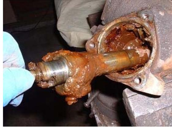
6. Remove the pitman shaft being careful not to lose the special shim on the adjusting screw.
