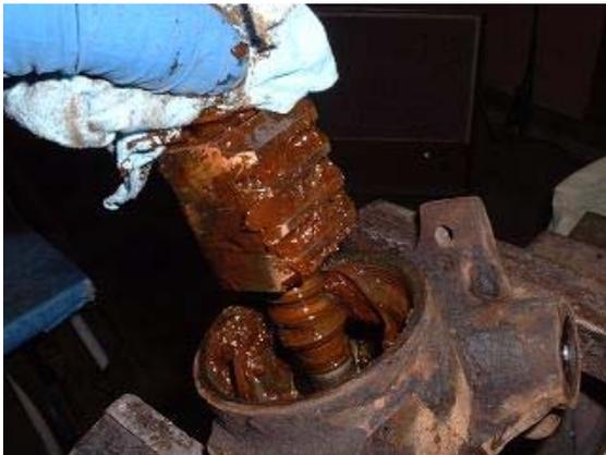
9. The worm gear and nut should pull out easily. That's why we cleaned and sanded the shafts. Now is a good time to clean out the old grease.
